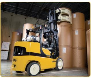
maintenance. The steering wheel is 30cm in diameter with a textured surface grip and spinner knob, and requires only four turns lock-to-lock. The centre mounted steer cylinder is located within the confines of the steer axle for protection.
